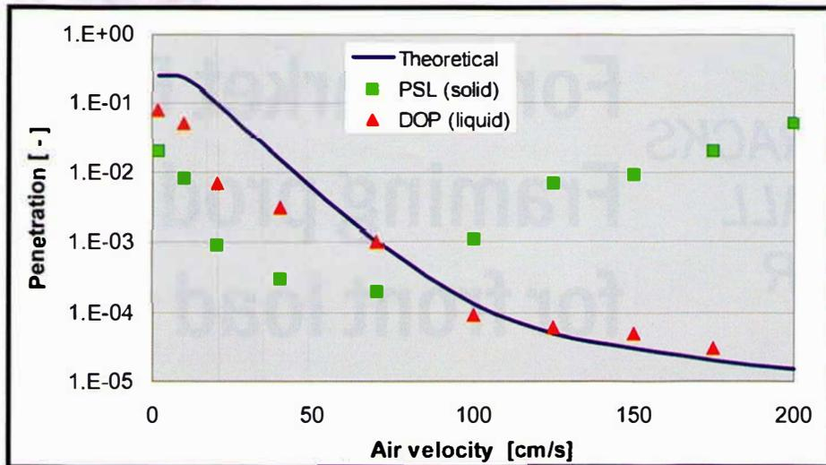
Figure 1: Experimental compared with predicted theoretical filter penetration for solid (PSL) and liquid (DOP) 2.0 µm particles according to [7]. Bouncing-off effect increases penetration of solid particles for higher air velocities.
